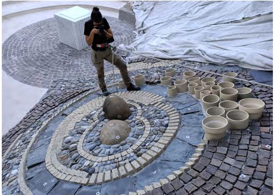
Figure 8 Acquisition campaign of the mosaic portion. The photos were taken with a Nikon D5300 camera, with an 18mm lens.
